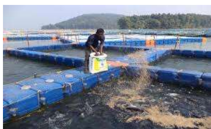
Fig 1: HDPE Floating Pontoon Cubes used for suspending Nylon Net Cages for fish
